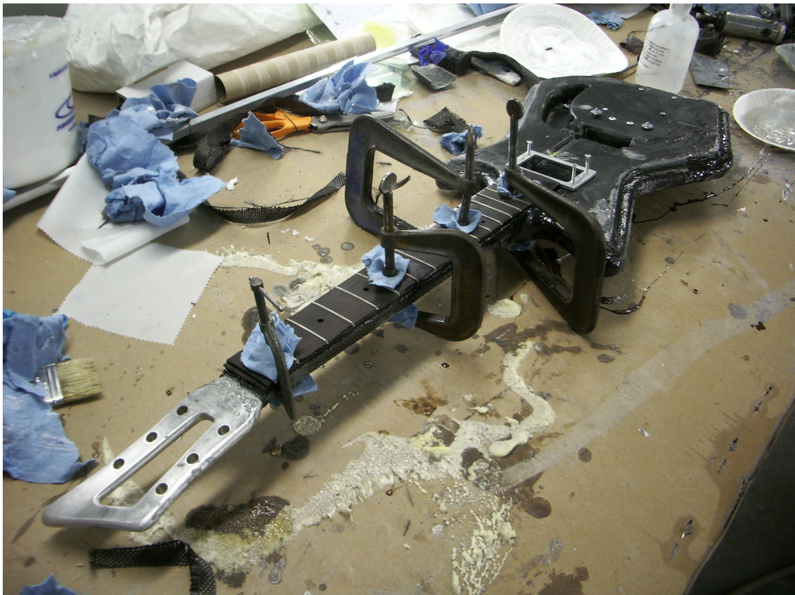
Figure 28. Attaching the Fretted Fingerboard
