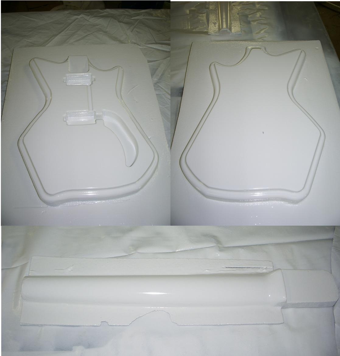
Figure 18. Second Layer of Duratec Surfacing Primer
