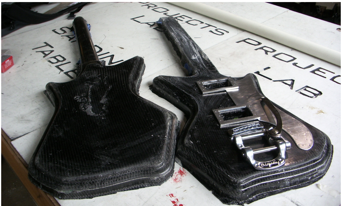
Figure 25. The Completed Carbon-Fiber Halves
