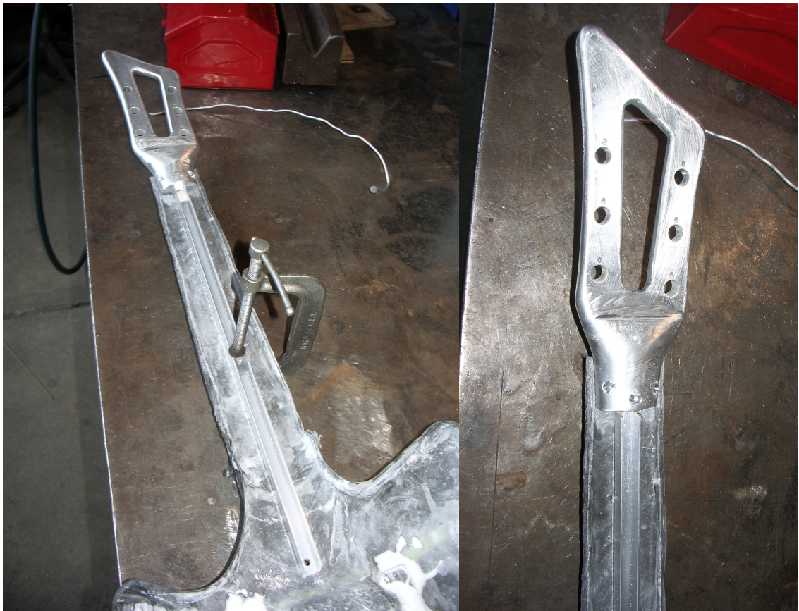
Figure 27. Aluminum U-Channel Riveted to Neck and Headstock
